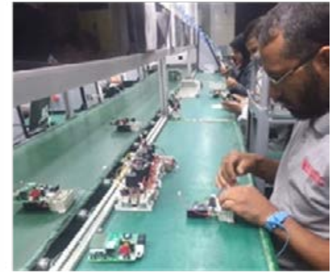
Assembly of the water meter
