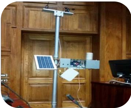
Model of Automatic Agriculture Weather Station
