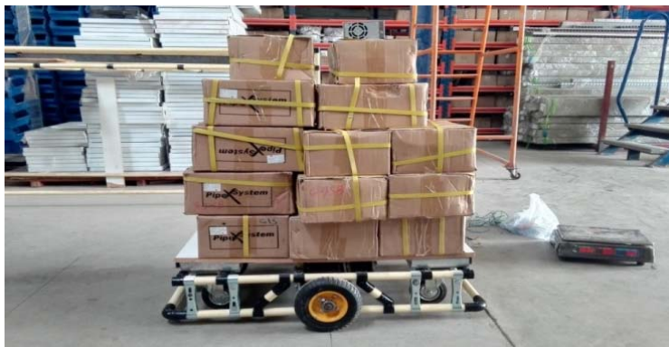
The produced AGV carrying 500 kg load
